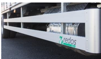
Tilting underride guards (anodized aluminium)
