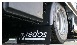
Mudguards with anti-splash mud flaps
