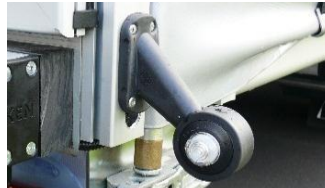
Outline marker diodes compliant with the EU Traffic Code
